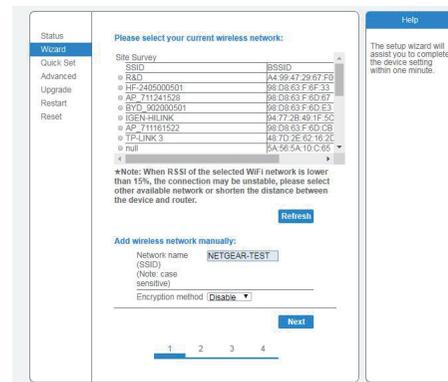
Notice: If the signal strength (RSSI) of the selected network is <15%, which means unstable connection, please adjust the antenna of the router, or use a repeater to enhance the signal.
